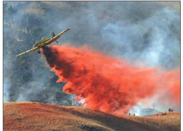
Single Engine Air Tanker (SEAT) dropping retardant
